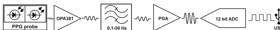
Fig. 2 Schematics of the PPG apparatus: a transimpedance amplifier (OPA381, Texas Instruments) based reflectance type PPG sensor with a photodiode (BPW34-FA, Osram, peak spectral response: 880 nm), an active 1st order feedback circuit 34 Hz low-pass filter, and the 875 nm LED (SIR91-21C/F7, Everlight, 400 mW, a transmission angle 20 deg, diameter 1.9 mm). The probe was connected to custom designed biosignal amplifier with an integrated band pass filter, consisting from 0.1 Hz 2nd order high-pass and 30 Hz 6th order low-pass filters.
